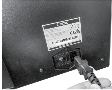
13. Take power cable out and plug it into power input.
