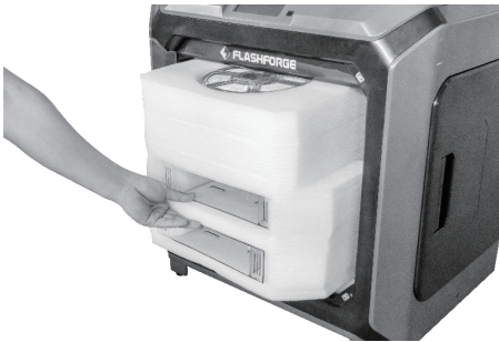
9. Open the front door and take out the front foam which should contain two filament spools and two waste boxes.
