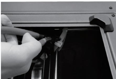
6. Take out the foam with accessories. Shear two ties on the both sides of X-axis guide rod.
