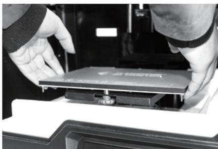
8. Hold both sides of the printing platform, and slowly lift the platform from the bottom to facilitate the removal of the foam box below.
