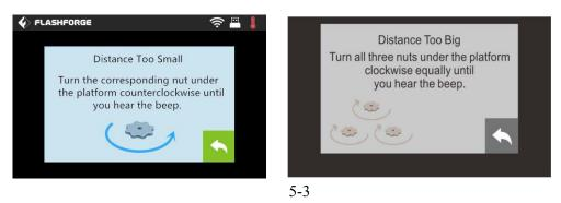
(5-3) When it shows that the distance is too small, please screw corresponding nut under platform counterclockwise; When it shows that the distance is too big, please unscrew all three nuts under platform clockwise; Until hearing a steady beep and the **[Verify]** button appears.
