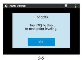
(5-5) Repeat steps 2 through 4 according to the prompts on the touchscreen to complete second and third points leveling and then Tap [Finish] to exit.
