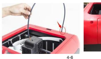
Next, we will load the FlashForge filament.(Note: Please lower the build plate to increase the distance between the nozzle and build plate to 50mm at least for avoiding nozzle jam.)
