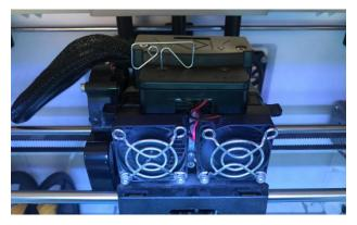
2.Clogged debris will be pushed down and will extrude from the extruder nozzle. You should push the unclog too all the way down to ensure all filament is purged. You do not need to push with excessive force, as this may damage the extruder.
