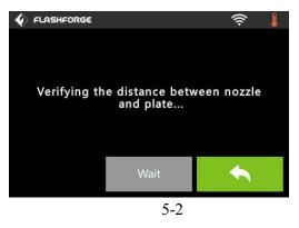
(5-2) After tapping **[OK]**, the extruder starts to move towards the first point and the plate moves up and down to verify the distance between nozzle and plate.
