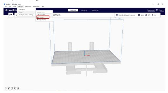
Option 2: On the main interface, click the Printer section, then click *Add printer* in the dropdown.
