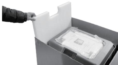
4. Remove foam around the printer.
