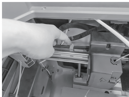
10. Remove clips on timing belt of X-axis and Y-axis.
